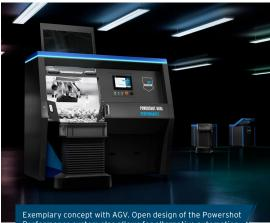
Exemplary concept with AGV. Open design of the Powershol Performance system also allows for alternative automation options such as robots, conveyor belts or similar.
